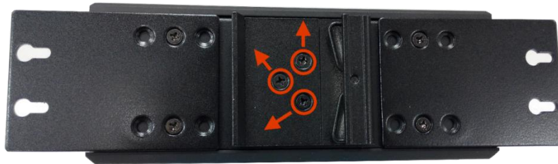
Figure 3.4: Remove DIN-Rail Bracket from the Switch
