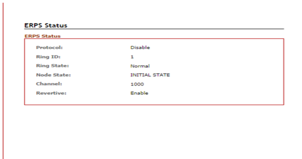
Figure 5.21 – Redundant Ring Network – ERPS Status
