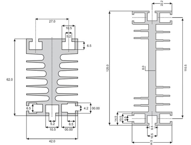
Fig 9 - Disipador ND10 (para 65mm: R<sub>thα</sub> = 2,0 °C / W)
