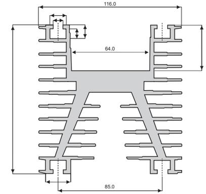
Fig 11 - Disipador ND40 (para 100 mm: R<sub>thα</sub> = 0,65 °C / W)
