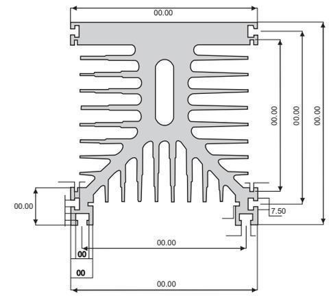
Fig 9 - Disipador NDP3 (para 120 mm: R<sub>thα</sub> = 0,52 °C / W)
