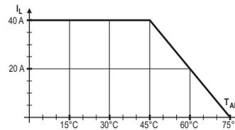
Fig 5 - SSR2540/4840 + disipador ND40-100 mm
