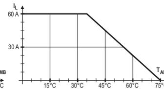
Fig 6 - SSR4860 + disipador NDP3-120 mm
